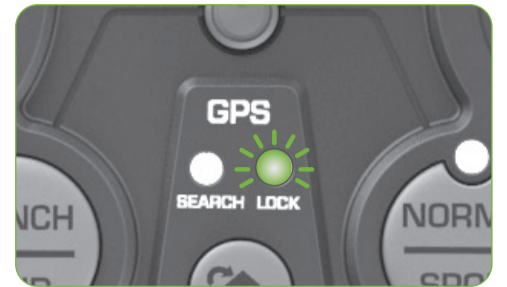
Once GREEN LOCK LED turns on solid, the drone is ready to fly.
